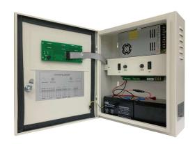
Auto boost-charge is triggered automatically when the battery falls below a preset voltage. An auto boost cycle can also be triggered manually via panel push-button. Once the batteries have reached the boost-charge voltage level, PSU series reverts automatically to its normal float charge mode, preventing battery over-charge.
