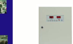
The PSU applies AC220V as its primary power and sealed lead-acid battery as standby power. In case of commercial power failure, it can automatically switch to standby power. Applying switched power voltage stabilizing circuit and standby power float charging circuit, it has the functions of automatic over-current protection, switch between primary and standby power, and automatic charge and over-discharge of standby battery.
