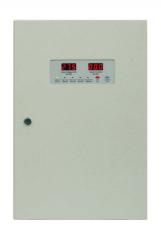
The PSU applies AC220V as its primary power and sealed lead-acid battery as standby power. In case of commercial power failure, it can automatically switch to standby power. Applying switched power voltage stabilizing circuit and standby power float charging circuit, it has the functions of automatic over-current protection, switch between primary and standby power, and automatic charge and over-discharge of standby battery.
