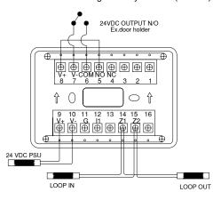
Wiring for 24VDC output
