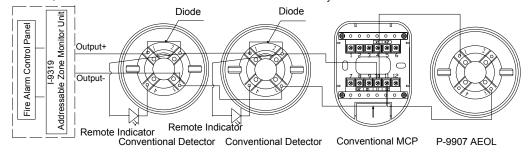
When the AEOL is not used as the detector base, a cover should be added, the system connection is shown below:
