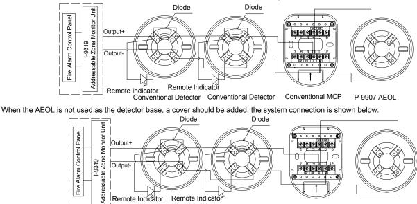
2. When the detector is connected with conventional fire alarm control panel (those within the dotted line are equivalent to a conventional fire alarm control panel) or I-9319 Addressable zone monitor unit in series, if an end of line resistor is connected to the end of output loop, then no diode is connected to the detector base. The system connection is shown below:
