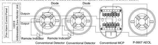
2. When the detector is connected with conventional fire alarm control panel (those within the dotted line are equivalent to a conventional fire alarm control panel) or I-9319 Addressable zone monitor unit in series, if an end of line resistor is connected to the end of output loop, then no diode is connected to the detector base. The system connection is shown below:
