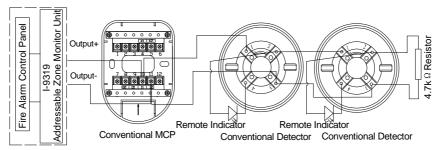
Maximum 15 detectors can be connected in one zone. Cooperating with end of line device, the compatible panel can monitor the cable for open circuit and short circuit. Panel will report if any detector is removed. With the AEOL, the functioning of other device will not be affected by the detector removal.
