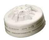
The Orbis I.S. Heat Detector monitors temperature by using a single thermistor which provides a voltage output proportional to the external air temperature.
