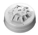
The Orbis Heat Detector monitors temperature by using a single thermistor which provides a voltage output proportional to the external air temperature.
