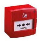
A seven-segment DIL switch enables the addressing of each call point at commissioning stage. When operated, the manual call point interrupts the polling cycle for a fast response. Bi-coloured LEDs indicate isolate and normal conditions.
