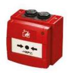
The Waterproof Manual Call Point has been designed for use outdoors and in places where moisture can occur. A seven-segment DIL switch enables addressing of each call point at commissioning stage. When operated, the manual call point interrupts the polling cycle for a fast response. Bi-coloured LEDs indicate isolate and normal conditions.
