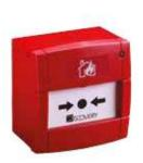
A seven-segment DIL switch enables addressing of each call point at commissioning stage. When operated, the manual call point interrupts the polling cycle for a fast response. Bi-coloured LEDs indicate isolate and normal conditions.
