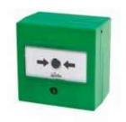
The Dual Switch Manual Call Point provides volt free double pole changeover contacts suitable for normally open or normally closed multiple switching from a single activation point. A device is activated by pressing the resettable element. An activation status is indicated through the rotation of the resettable element, displaying yellow and black indication bars. The manual call point can be easily reset from the front using the supplied reset key.
