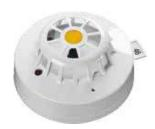
The XP95 Heat Detector monitors temperature by using a single thermistor which provides a count output proportional to the external air temperature. The XP95 range features two heat detectors, standard and high temperature. The standard heat detector is classified as an A2S device and will report an alarm at 55°C. The high temperature detector, classified as a CS device, will report an alarm at 90°C.
