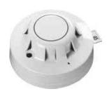
The XP95 Ionisation Smoke Detector uses a low activity radioactive foil to detect fires by irradiating the air in the smoke chambers and causing a current flow. If smoke enters the chamber, the current flow is reduced leading to an alarm.
